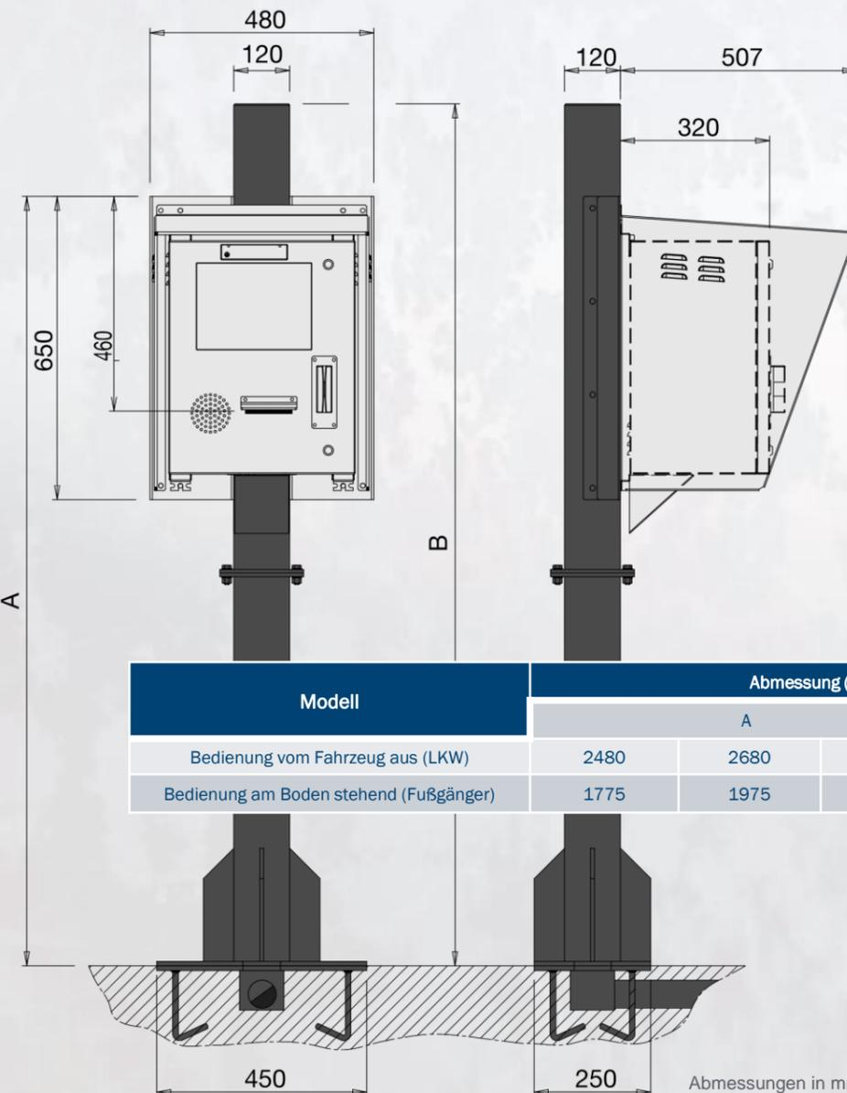
Abmessungen in mm
